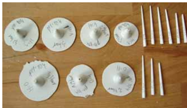
Low-pressure injection-molded cones (on the left) and needles (on the right) from paraffin suspensions of coated alumina at pH 10.4, before (upper line) and after (bottom line) the addition of water. In spite of water being added to the suspension of coated powder, the rheological properties remained suitable for low-pressure injection molding, moreover, the quality of injection-molded parts remained unchanged.
