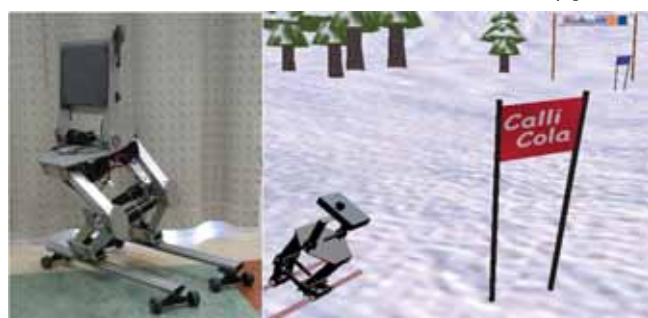
Figure 3: Robot skier mechanism and simulation of skiing in a virtual environment
