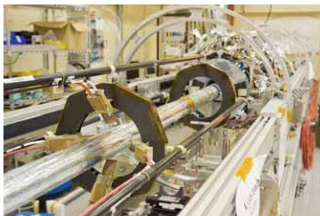
Figure 1: Four detector modules of the ATLAS Beam Conditions Monitor installed in the support structure of the pixel detector. The 72-mm-diameter beam pipe can be seen, as well as the pixel detector in the background.
