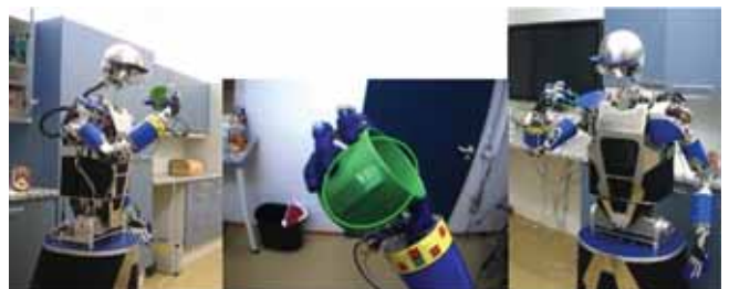
Figure 1: Object learning on the Armar III humanoid robot (Experiments made at the University of Karlsruhe)
