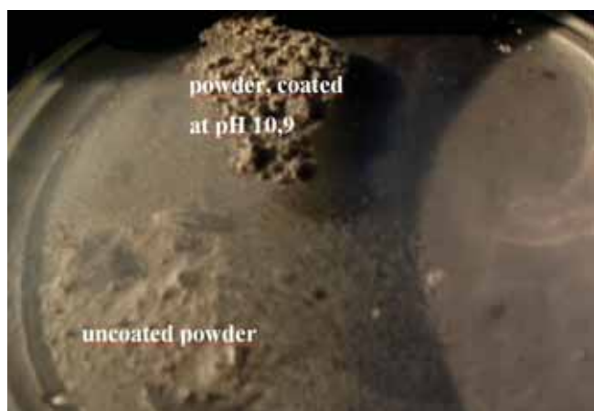
Photograph of coated and uncoated \text{Al}_2\text{O}_3 powder in a petri dish with water. In contrast to the uncoated powder, which is easily wetted, the coated powder (at pH 10.9) floats on the water's surface.
