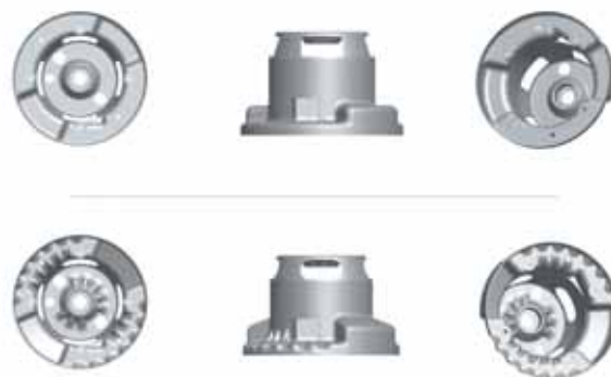
Figure 1: Electrical-motor case: (upper) initial and (bottom) optimized, where its geometrical shape was optimized and the original stiffness kept for a 20% thinner material.
