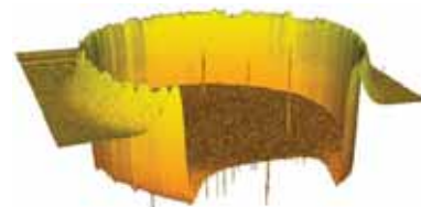
Figure 1: Surface topography of a crater, prepared by glow-discharge optical spectrometry (picture width is 5 mm, crater depth 5 \mu\text{m} )
