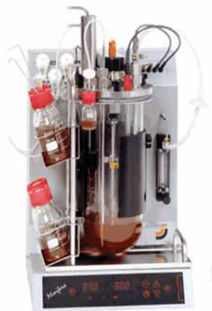
Figure 1: The optimisation of brazzein expression was performed simultaneously in four fermentors Minifors (ATR Biotech).
