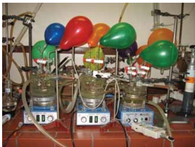
Figure 3: Reaction vessels for an aerobic oxidative iodination of organic compounds. In green chemistry the most favourable oxidant is air at ordinary pressure. The balloons serve as oxygen reservoirs for the chemical reaction of oxidation and, at the same time, variegate the laboratory.
