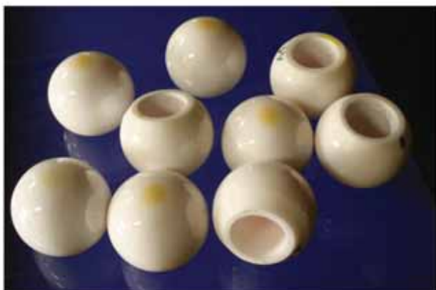
Figure 2: Test series of ceramic ball-heads for hip joints with a gradient composition were produced in the frame of the European project "Biograd". ( http://cordis.europa.eu/fetch?CALLER=OFFPR_TM_EN&ACTION=DEDOC=2&CAT=OFFRE&QUERY=1197645527573&RCN=3420 )
