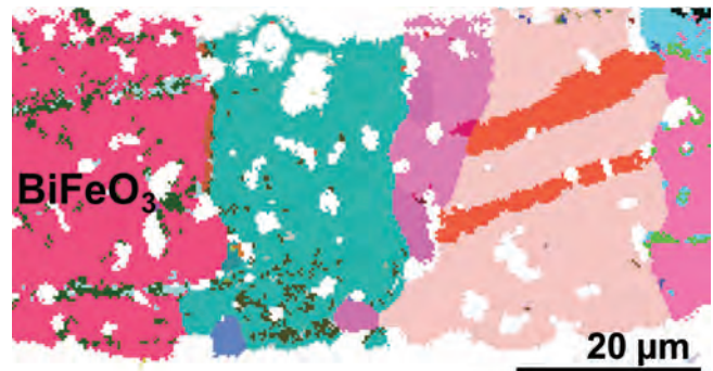
Figure 3: Distribution of the crystallographic orientations in columnar grains in thick \text{BiFeO}_3 film with pronounced domain structure.
