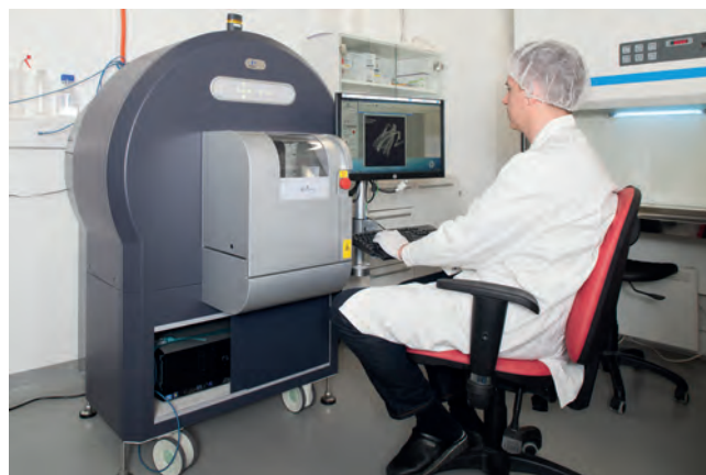
Figure 1: Quantum FX micro CT apparatus (Perkin Elmer) enables CT imaging of small rodents in preclinical investigations
