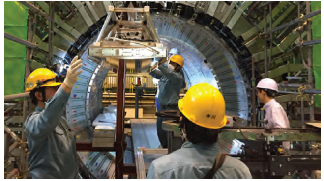
Figure 3: Placement of quartz radiators for Time-Of-Propagation counter
