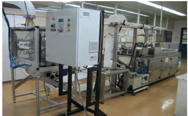
Figure 9: An atmospheric pressure plasma reactor was integrated to the production line at Tosama company for the deposition of antimicrobial thin films on wound care products in the frame of the European project IP4Plasma
