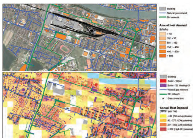
Figure 3: Spacial analysis of heat use in the area of Maribor: annual heat use in buildings, space density of heat use, types of heating appliances and energy infrastructure (distribution network of district heating and natural gas).
