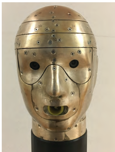
Figure 6: Sweating thermal head manikin
