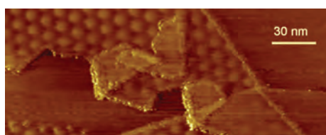
Figure 27: STM picture of a superstructure in graphene lying on graphite substrate.
