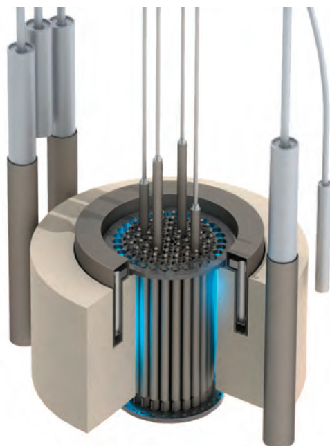
Figure 2: Photorealistic schematic of the TRIGA reactor where the core, graphite reflector and ex-core detectors are depicted.
