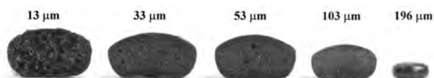
Figure 7: Cross-section images of the foam glasses prepared from panel glass powders with different particle sizes. The density of the foam glass prepared from 13- \mu\text{m} powders is 120 \text{kg}/\text{m}^3 .
