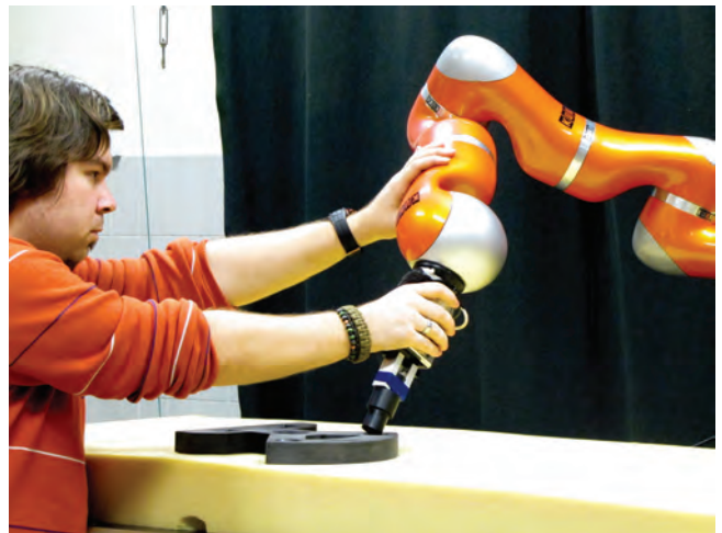
Figure 3: Robot programming by kinesthetic guiding
