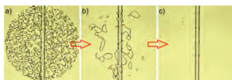
Figure 20: During the fast quenching of a liquid crystal from isotropic to nematic phase tangle of defect lines appear (a) and two pairs of Saturn rings and anti-rings are formed around the glass fibre (c).
