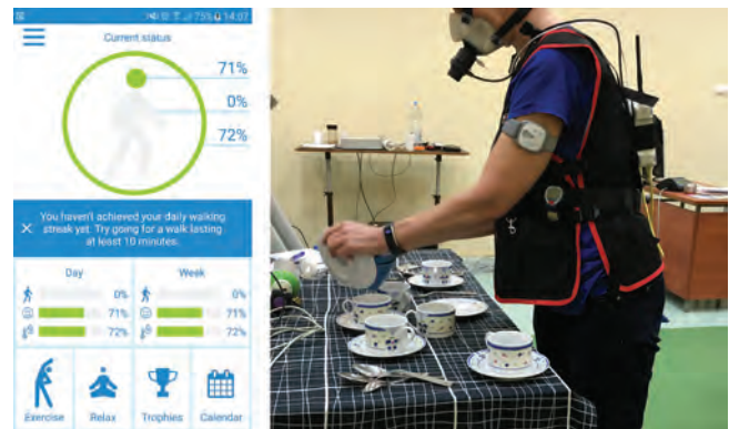
Figure 4: Fit4Work application, which helps older workers relax, be physically fit and have a good work environment (left). Measurements of human energy expenditure needed to develop the application (right).
