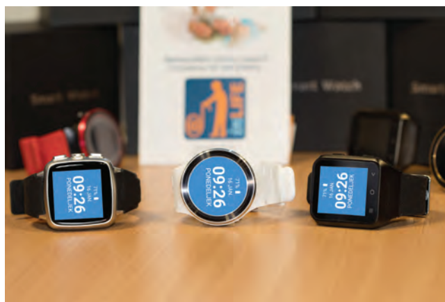
Figure 1: Within the framework of the H2020 IN LIFE project we developed a smart watch for the elderly and prepared 150 pieces for a 6-month-long pilot testing. The watch allows around 10 functions, including calls to the carer, automatic fall detection, location identification and call for help, notifications, monitoring of physical activity, etc. The system is a personal assistant and carer for the elderly. Our vision is to introduce it to the care of the elderly Europe-wide, thus increasing the quality of life.
