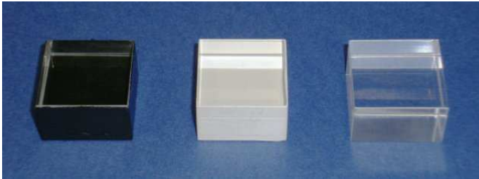
Figure 4.7: Black painted, Teflon wrapped and bare \text{PbF}_2 crystals with dimensions of 25 \times 25 \times 15 \text{ mm}^3 .
