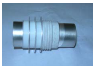
Fig.3: Electron gun assembly and its demountable UHV assembly with 95 GHz FW-BWO [5]
